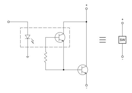
Figure 5.3 Isolated Loop Current Switch
