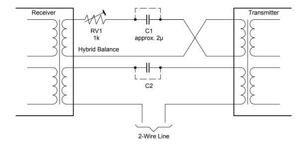
*Figure 4.3 4-Wire to 2-Wire Converter*
