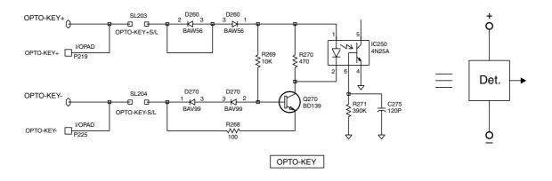
Figure 5.2 Isolated Constant Current Loop Current Detector (Opto-key input on T836 & T837)
