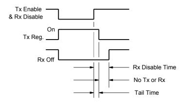
Figure 4.4 Receiver Disable Time vs Tail Time
