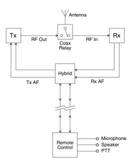
Figure 4.2 Remote Line Controlled Base Station
